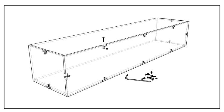
Slide the nut to one if the slot of the T joints, place the screw form the top and tighten it gently.
