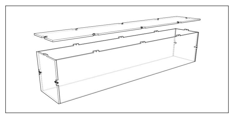
Place the top panel, and turn the box to one of its side.
